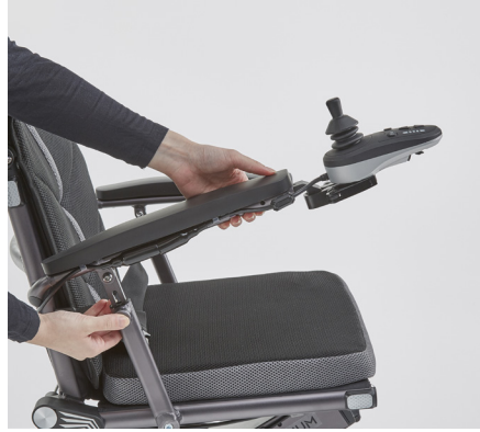
Step 2: Press the unlock button while pulling the armrest up
