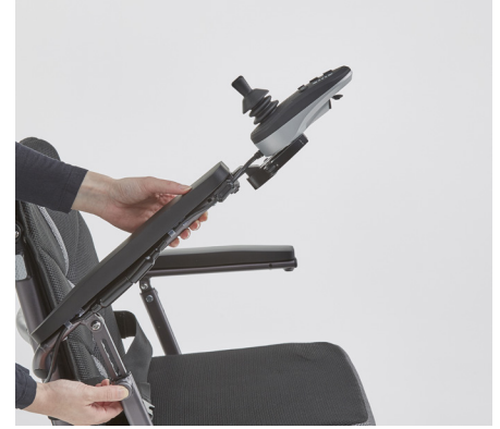
Step 3: Pull the armrest to the extreme position.
