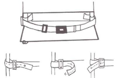
The Shoulder Straps 'slide-fix' to the tubular handles of the wheelchair & loops on to each side of buckle
