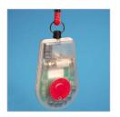
TIR4 infra red trigger – designed to be worn by residents or staff and enables calls to be generated remotely from the call point. This is ideal in lounges or common rooms where each resident can be given a trigger to allow access to the call system. The TIR4 requires an infra red enabled call point to operate (such as an L722 or an L752). When using the TIR4 with an integral 700 system, it is possible to identify the call location and the individual caller.
