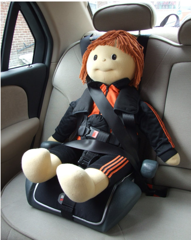
Illustrating one of our harnesses fitted in conjunction with the existing vehicle safety belt.
