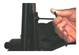
The height of the footrest is set by loosening the grub screw on the back of the footrest bracket.
