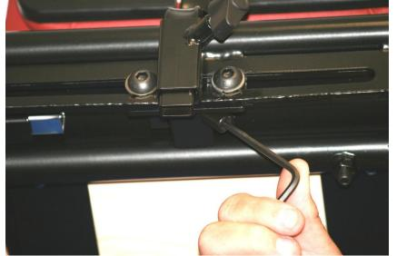
the seat by adjusting the hip guides. The width between the hip guides is set by loosening the grub screw beneath the seat as shown. The hip guide mounting can then be moved outwards and the grub screw retightened.
