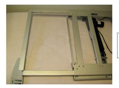
With the trombones adjusted to fit the bed, there is a gap between the width adjusting trombone and the central frame section.
