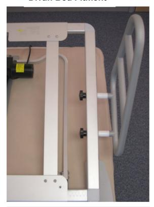
When fitting the Side Rail for a divan bed, the plastic spacers should be put onto the threaded rods before they are introduced to the trombone. The hand wheels should then be tightened against the inside of the trombone until a firm fitting is achieved. This will allow the rail to be on the outside of the mattress.
