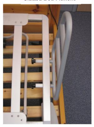
When fitting the Side Rail for a slatted bed, the threaded rods should first be introduced to the trombone, then the plastic spacers put onto the rods and finally the hand wheels tightened until a firm fitting is achieved. This will allow the Side Rail to fit inside the frame of the bed in its lowest position.
