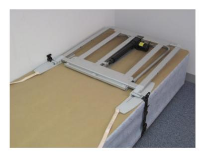
4. Connect one of the 2.5m brown straps to the lower female buckle from the strap bracket at one side of the bed. Pass the long strap under the bed and connect at the other side. Tighten the strap to secure the elevator to the bed base, then tidy away any excess strap to avoid a trip hazard.
