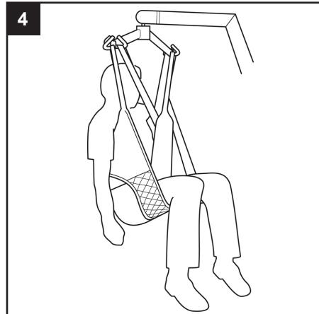
Cross over the leg straps and attach to the spreader bar on the front hooks using the longest loop. Raise the hoist and attach your desired shoulder loop to the rear hooks (a more upright position will be achieved using the shortest loop).
