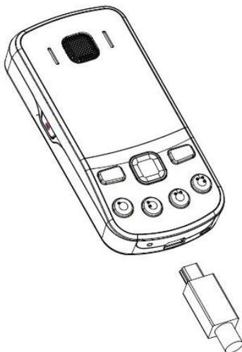
Next, connect the charger to an AC wall socket. A message on the screen will confirm that the charger is connected. The battery charge level indicator at the top right of the screen will indicate the Oysta Pearl+ is charging.
