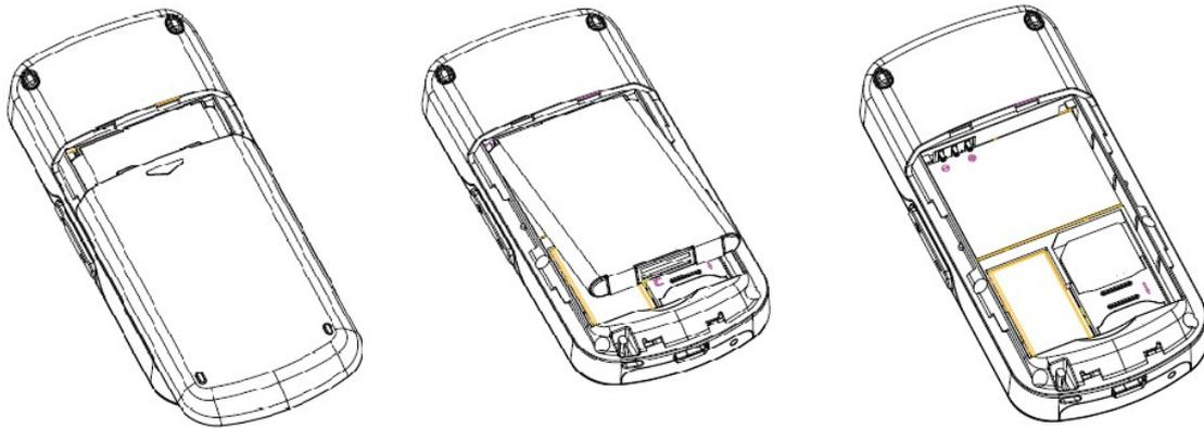
Close the SIM card holder and move it to the right to lock. Slide the battery back in and push it down to lock it into position. Next, place the back cover back in place.
