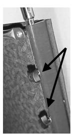
The push handles are fitted to the wheelchair when it is delivered. To adjust the height to suit you, simply unscrew (*turn anti clockwise*) the two thumbscrews at either side and near the top of the backrest. (*See photo opposite*) Lift or lower the push handles to a height that suits you then retighten (*turn clockwise*) the thumbscrews.
