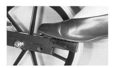
To tip the wheelchair backwards when climbing kerbs stand behind the wheelchair holding onto both push handles. Place one foot, either the right or left, whichever suits you, onto the tipping lever as shown in the picture opposite. Press down with your foot and pull back with your arms. The front of the chair will lift.
