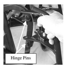
To fit the right hand footrest, stand in front of the wheelchair. Remove the spring clip from the lower hinge pin on the side of the wheelchair. Making sure the footplate is facing in towards the centre of the wheelchair place the footrest onto the hinge pins. (See Photo opposite). Replace the spring clip. Swing the footrest towards the centre of the wheelchair until it locks in place.
