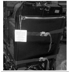
Left: The backboard correctly fitted to the back of the chair.
