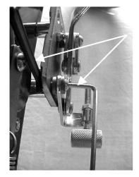
To move the brake assembly use a 3 mm hexagon key and 8 mm spanner to remove the rear brake linkage screw making a note of the position of the spacers. (See photograph below).
