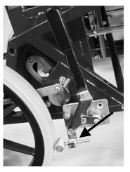
Adjust the brakes by loosening the nut (*arrowed*) locking the brake pad in place. Turn the brake pad so that it is near to, but not touching, the tyre. Retighten the locking nut.
