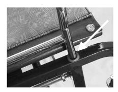
Standing at the side of the wheelchair place each armrest into the holes in the wheelchair frame. (*See photo*). Make sure they are pressed into the wheelchair frame properly.
