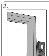
Remove the screw caps & Secure the monitor to the door frame or adjacent wall using he screws provided.
