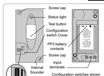
1. Install a 9 volt PP3 alkaline or lithium battery making sure to observe the correct polarity.
