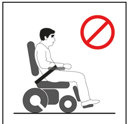
Figure 4.20: Wrong position hip belt
