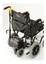
This wheelchair is suitable for some retrofit powerpacks, such as the PowerStroll. A suggested configuration is shown left.
