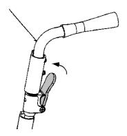
Push the black paddle (arrowed) towards the back post with your thumb whilst pulling the handle down. Repeat this operation for the other handle. To put the backrest back into position, lift both handles together and the folding mechanism will lock back automatically.
