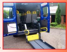
Entry is through a full height side door which gives easy passenger access. A variety of tail-lifts is available for wheelchair and disabled access at the rear of the vehicle.
