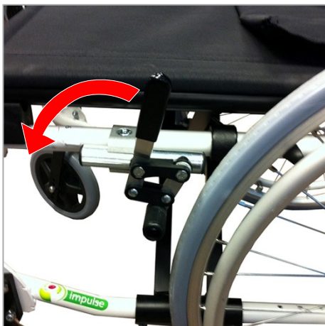
Figure 13: Push lever to apply brakes
