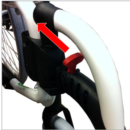
Figure 7: Pull back release lever
