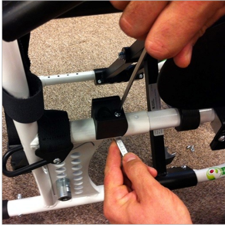
Figure 1: Remove nut and screw
