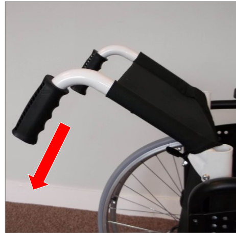
Figure 4: Fold down by pulling on handles
