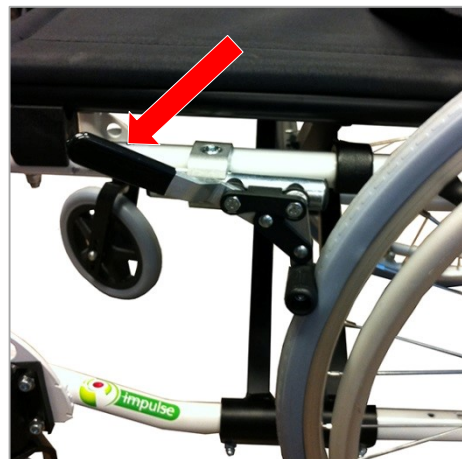
Figure 14: Push lever until it grips the tyre
