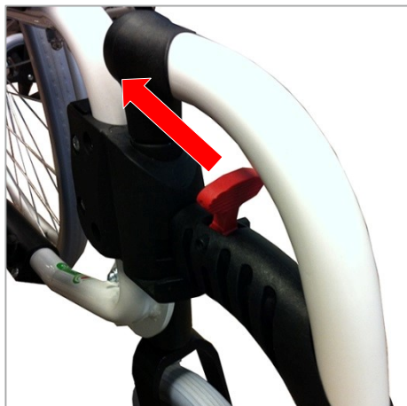
Figure 5: Pull release latch
