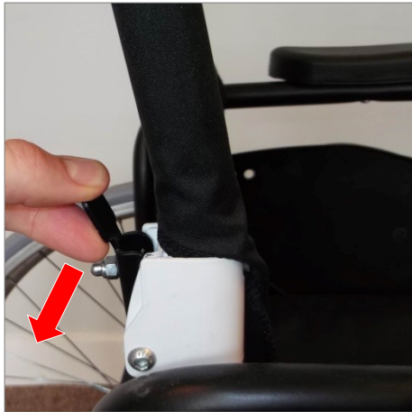
Figure 3: Push in black lever
