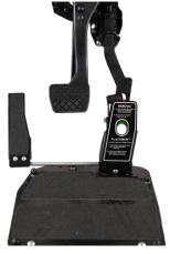
Brig-Ayd's Seat Runner Mounted Pedal Transfer allows the driver to operate the accelerator with their left foot, while the right is protected by a pedal guard.
