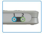
To adjust the trigger sensitivity for Channel 1 or 2, press the corresponding switch (1 or 2) then adjust using the Plus or Minus Switches.
