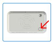
Press the Power Switch on the Patient Unit to turn on the device. The power LED will momentarily flash yellow, then periodically flash green to indicate the device is on.
