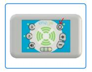
Press the Power Switch on the Base Unit to turn on the device. All LEDs will momentarily flash, then the green power LED will illuminate to indicate power on.
