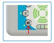
If audio feedback is required whilst adjusting the sensitivity, press the audio button until the desired mode (data/beep/off) is selected. While the audio LED is illuminated the volume can be adjusted with the Plus and -Minus Switches.
