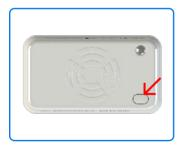
To turn off the Patient Unit hold down the Power Switch for 1 second then release. Patient unit will power down automatically after 5 minutes if there is no wireless signal from the Base Unit, or if placed on the Base Unit wireless power transmitter, or if the internal battery is too low.
