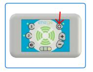
To turn off the Base Unit press the Power Switch then release. If the USB cable is plugged in, the Base Unit will be in stand-by mode and the Patient Unit can still be charged.
