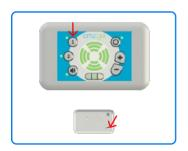
Press the Channel 1 or 2 Switch to connect the Patient Unit to the corresponding channel. LEDs 1 or 2 flash (briefly) when connected.
