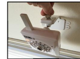
Plug the power cord into the back of the camera. Wrap the cord loosely around the bracket so it does not pull on the camera. Then plug the camera power adapter into the wall outlet.
