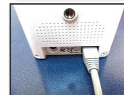
Insert the round plug from the supplied AC power adapter into the back of the camera.
