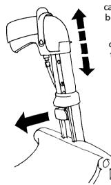
By pulling the orange-coloured button you can adjust the height of the handles to between 100 and 76 cm.
