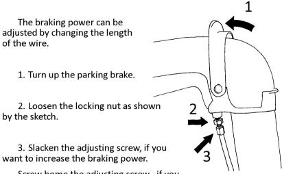
Screw home the adjusting screw , if you want to reduce the braking power.
