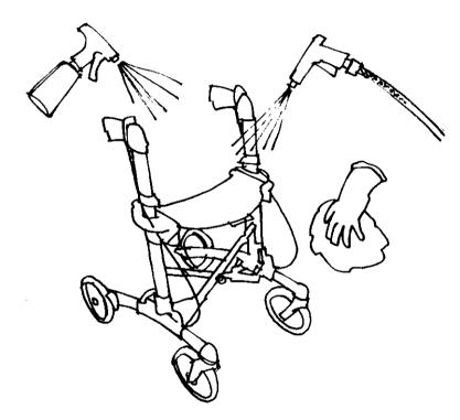
Make sure that no dirt is gathered between the wheels and the brake shoes. Dirt might jeopardize the braking power.
