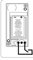
A short circuit between terminals 1 & 3 will activate the monitor if configuration key 7 is set.
