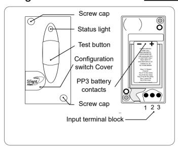
1. Install a 9 volt PP3 alkaline or lithium battery making sure to observe the correct polarity.
