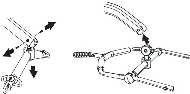
Once the standard fixing bolts are removed, connecting or disconnecting either system thereafter is completed easily by the use of a quick-release pin included with the shallow 4-point cradle. This is done quickly and easily, but you must read the following safety instructions to ensure the shallow 4-point positioning cradle/spreader bar is safely locked into position before use.
