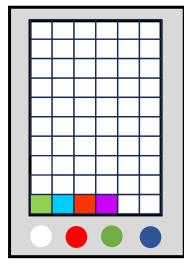
Individual Squares, the display showcases a dynamic visual effect where individual squares of colour increase in size in response to the detection of noise. As sound is heard, each square on the panel begins to expand, growing larger and more vibrant with each noise detected.
