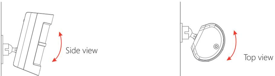
**Note:** If used in a pet friendly environment, for best results keep the PIR parallel to the wall, do not tilt it up or down.
