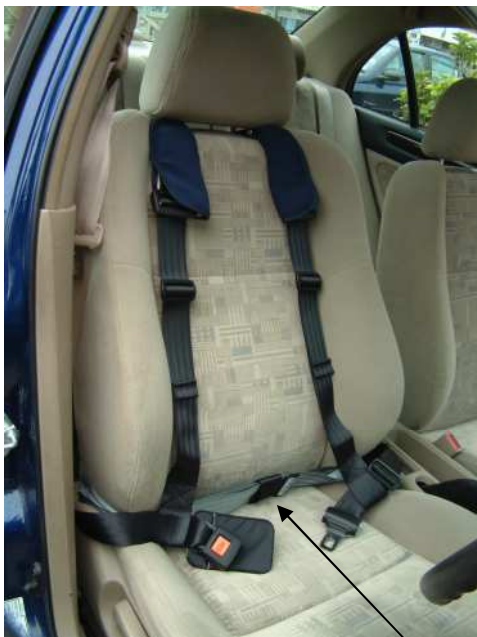
Inner Chair Strap fitted with Duraflex Side Squeeze buckle
